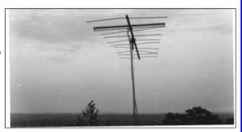
we had a 6 element yagi on 6m, four 2m antennas in a loose H-frame, and a single yagi on 220MHz. Our set-up was fairly easy--the biggest task seemed to be pushing
